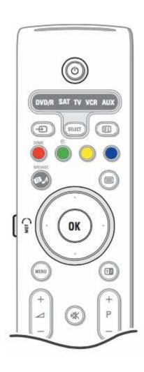
Select button switches between the device being controlled (flashes green):
